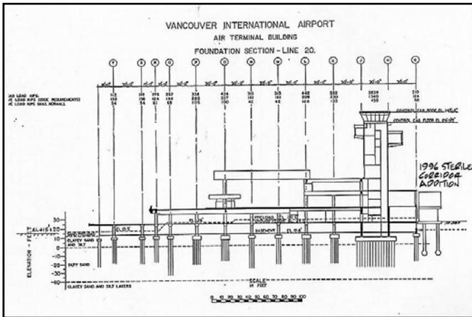
Figure 2 Section through DTB prior to seismic upgrade
