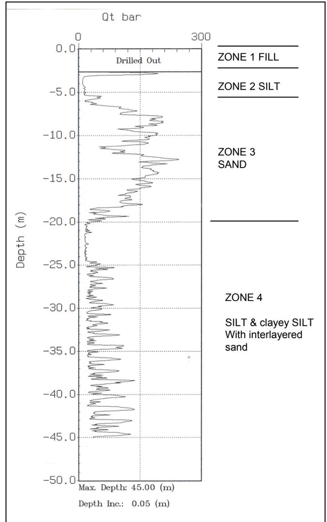
Figure 3 Soil Profile with typical CPT log
