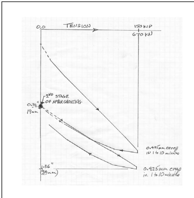
Figure 7 Micro-pile where second stage of after grouting was required due to excessive elongation of initial tension proof test
