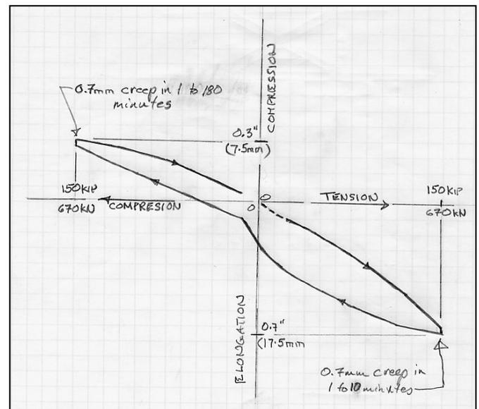
Figure 6 Tension-compression test on micro-pile
