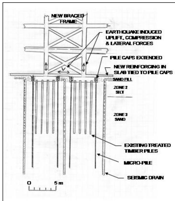
Figure 4 Schematic key seismic upgrade features
