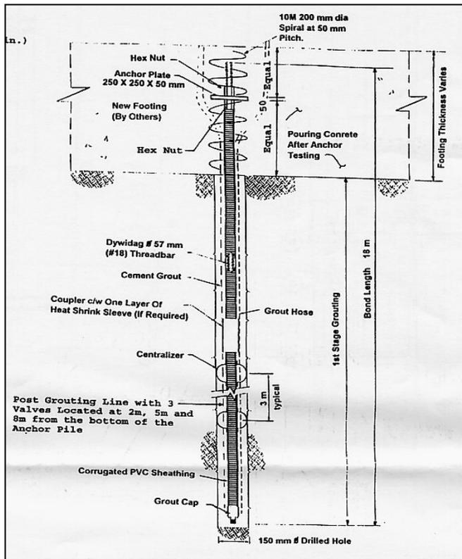
Figure 5 Typical micro-pile detail
